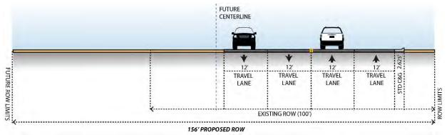
Figure 6: Paseo del Norte – Approximately 850-ft west of Kimmick Drive to Calle Norteña **Typical Section 4**
